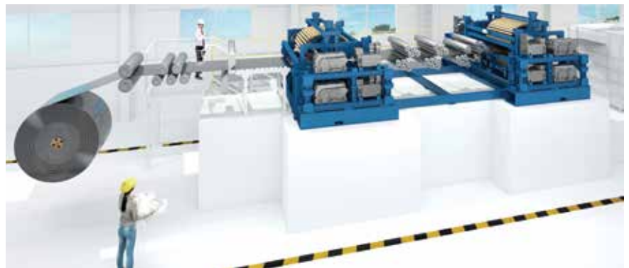
SDI's push-pull pickle line in Columbus will be the first in the world to operate with three Umlauf Bridles
