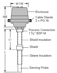
HEAVY PROBE WITH INTEGRAL SWITCHING UNIT
