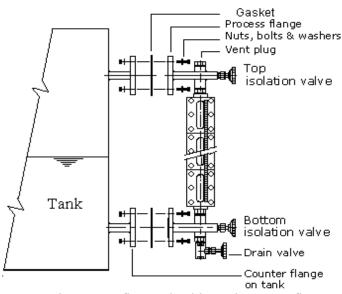
$\underline{\text{Note}}$ : \* Counter flange should match Process flange
